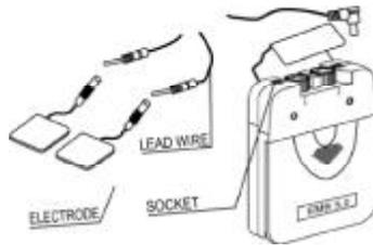
After connecting the wires to the stimulator, attach each wire to an electrode. Use care when you plug and unplug the wires. Jerking the wire instead of holding the insulated connector body may cause wire breakage.
