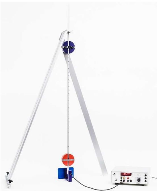
Fig. 5: Experiment set-up with light barrier and digital counter
