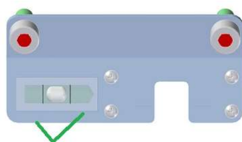
Fig. 3: Setting position with the help of the spirit level
