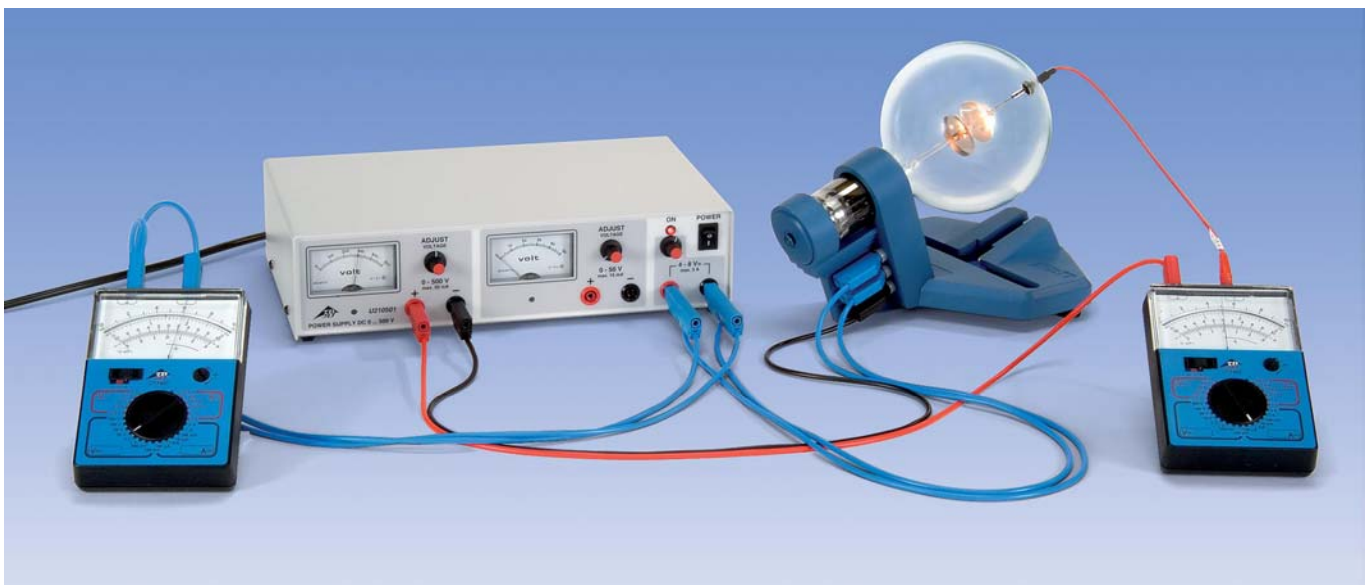
Fig. 1: Circuit (above) and experiment set-up (below) for recording the characteristic of a thermionic diode for different cathode heater voltages (1) Cathode, (2) Anode
