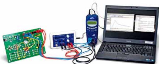
Measurement of the discharge of a capacitor
