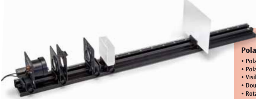
Visibility of polarised light in turbid water
