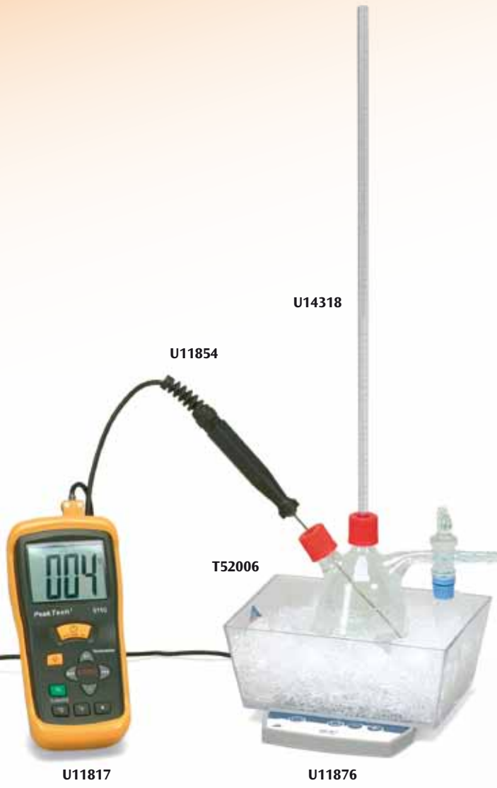
Determining the maximum density of water
