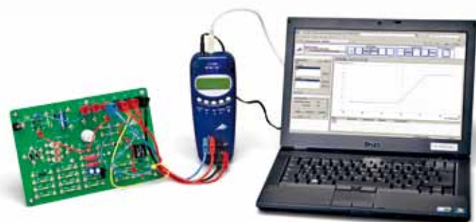
Characteristic curve for a zener diode
