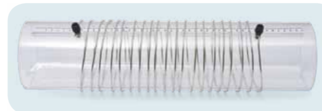
Fig. 1: Coil with variable number of windings per unit length
