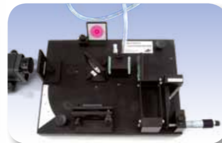
Vacuum chamber in the beam path of the Michelson-interferometer.
