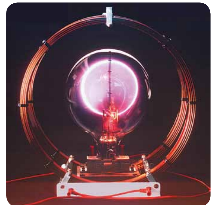
Fig. 2: Fine-beam tube with spherically-shaped luminous trace of electrons in the magnetic field
