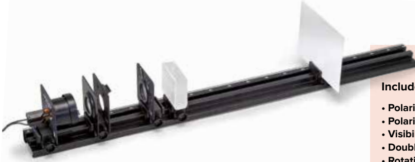
Visibility of polarised light in turbid water
