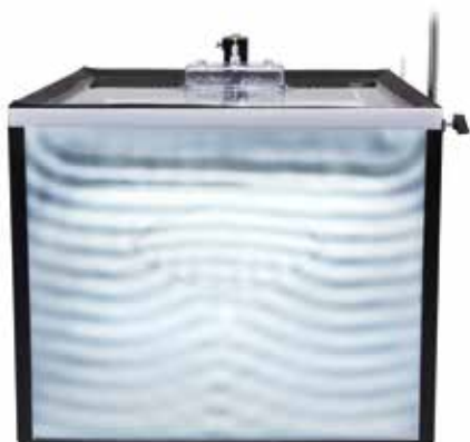
Refraction of water waves at a converging lens
