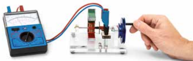
Operating as a DC generator
