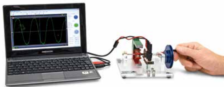
Operating as an AC generator
