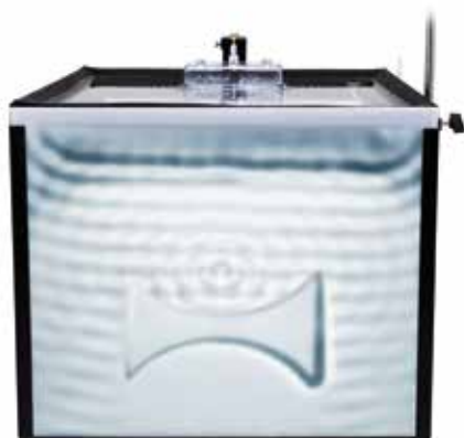
Reflection of water waves at a "concave mirror"
