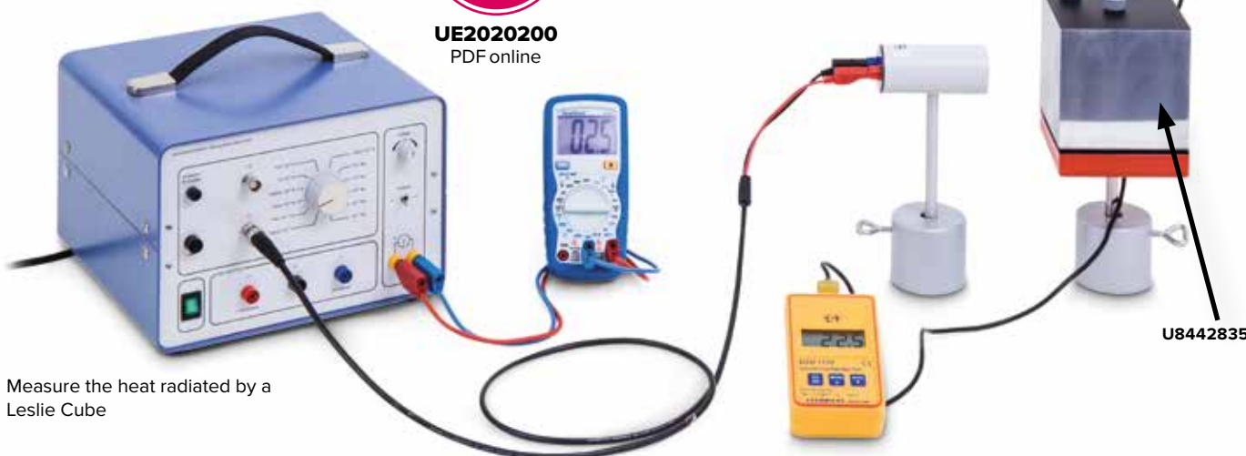
Radiated intensity from a Leslie Cube as a function of x = T^4 - T_0^4
