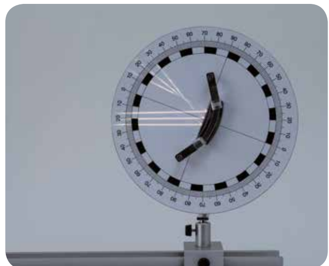
Fig. 3: Reflection of three parallel rays by a concave mirror
